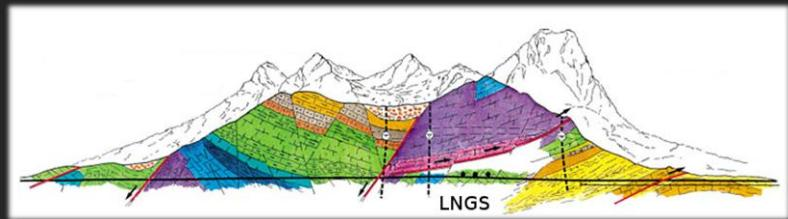
Natural coverage by the Gran-Sasso mountains provides the required shielding from the Cosmic rays.
