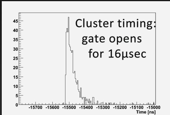
PMT time-of-flight distribution used for position reconstruction
