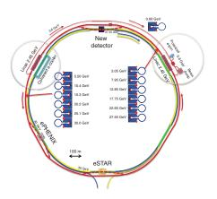
$\label{eq:error} \mbox{eRHIC at BNL} \\ \mbox{add } e^- \mbox{ LINAC to existing RHIC complex}$
