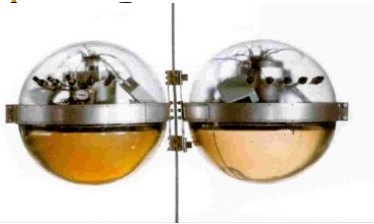
Quasar photodetector ( \varnothing=37\text{cm} )
