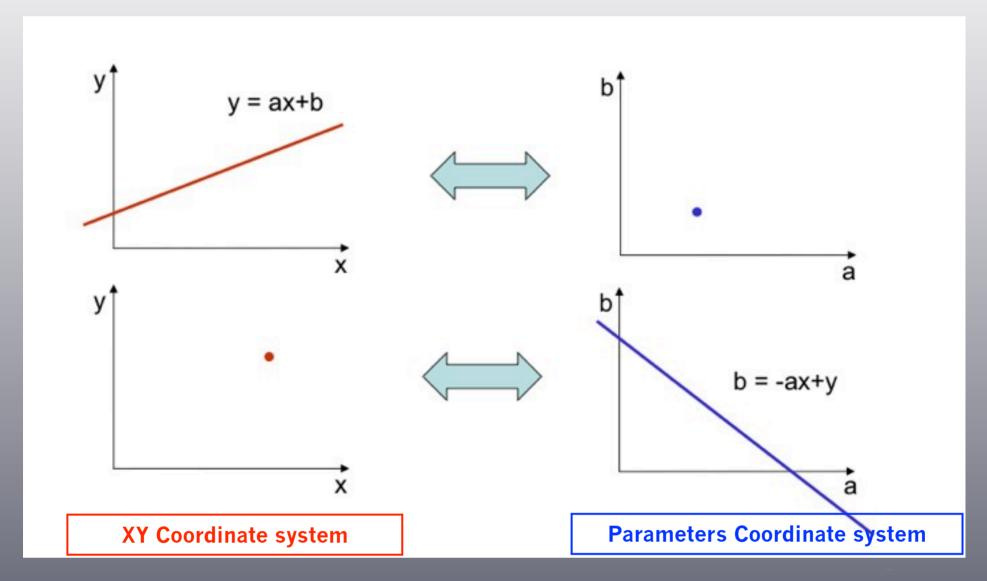
For each point (x,y), all the possible lines going through it are represented by a single line in (a,b) space
