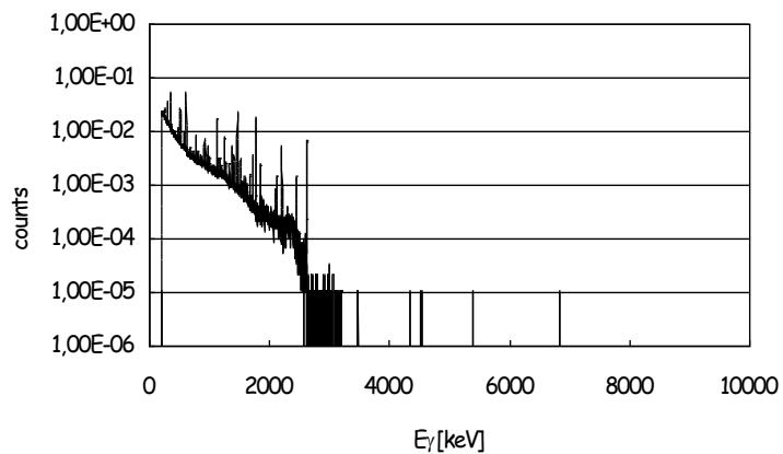
$E_{\gamma} < 3\text{MeV} \rightarrow$  passive shielding for environmental background radiation
