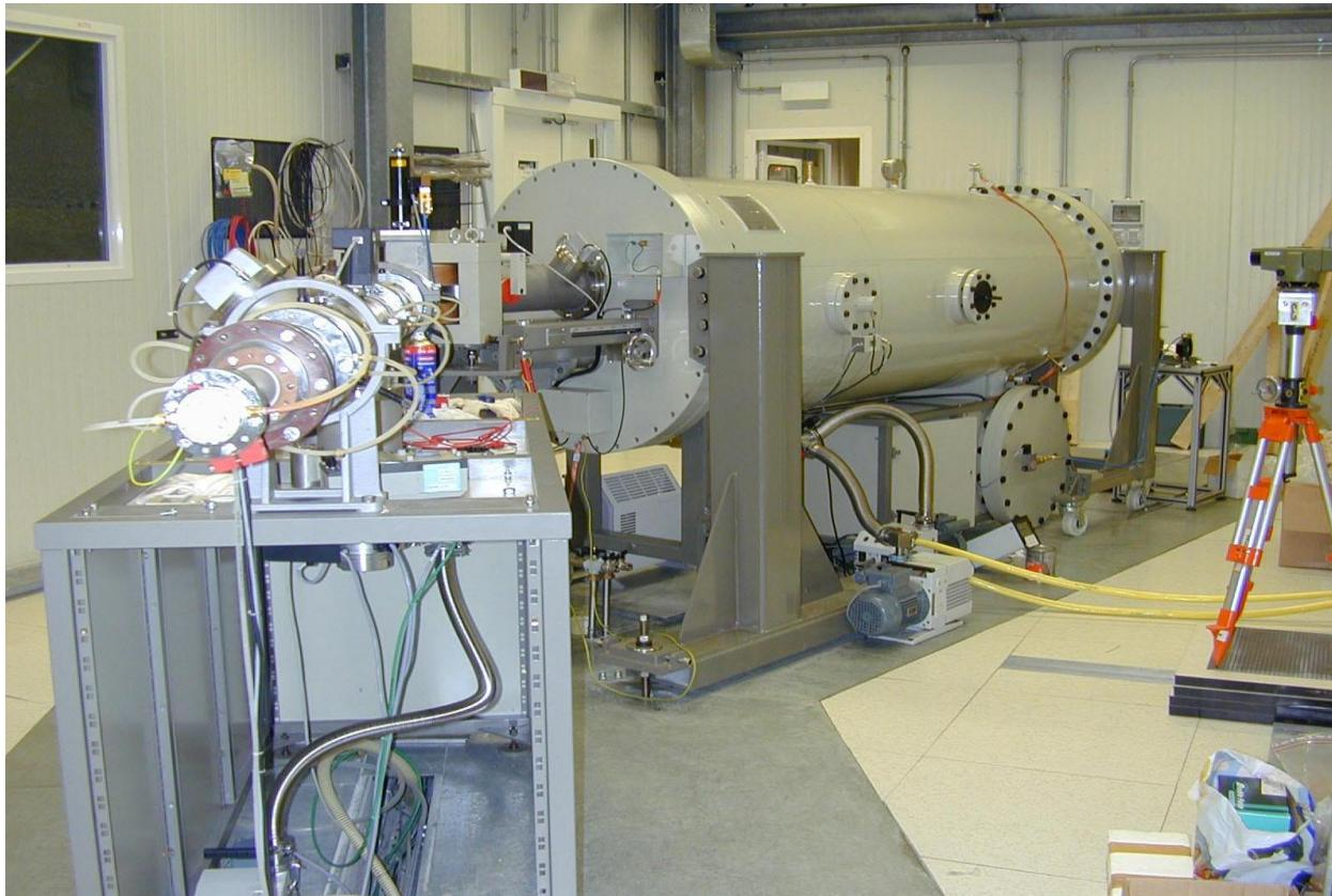
400 kV Accelerator :  $E_{beam} \approx 50 - 400 \text{ keV}$
