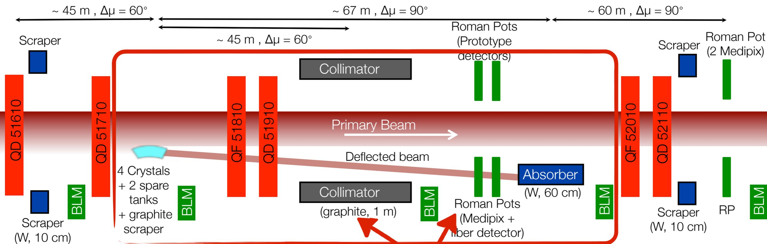
equipment for the measurements of the multi-turn halo (**upstream the crystal**)
