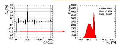
Observation: The effect of the lost DAC values is significant 0.2% for channels in EMB1.
