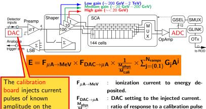
detector cell, in order to probe the actual electronic response
