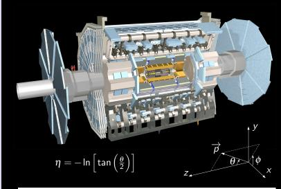
An electron is reconstructed as a track in the inner detector matched to a cluster in the calorimeters
