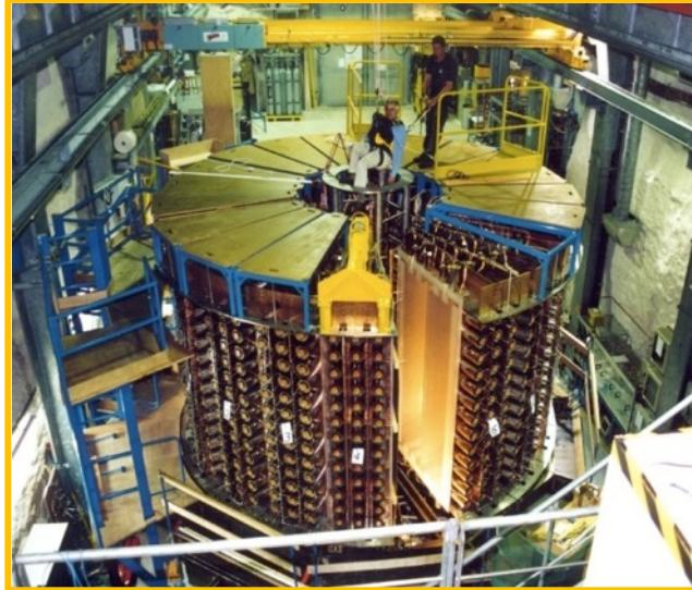
Tracking detector: drift chambers (6180 Geiger cells)
