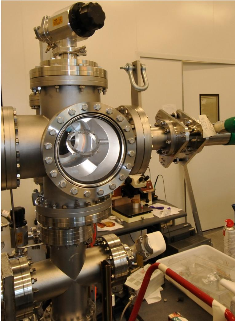
Production of FID detectors performed @ CSNSM-Orsay in a dedicated evaporator.
