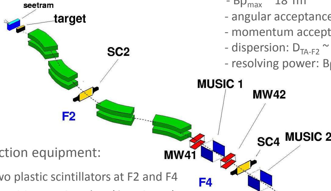
Two-stage, zero degree achromatic spectrometer:
