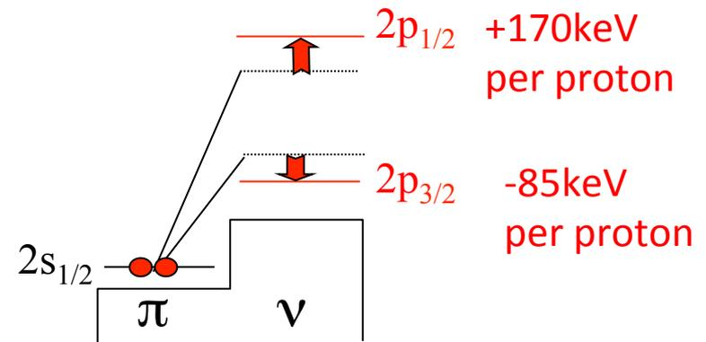
Increase of the SO splitting due to the two-body SO interaction
