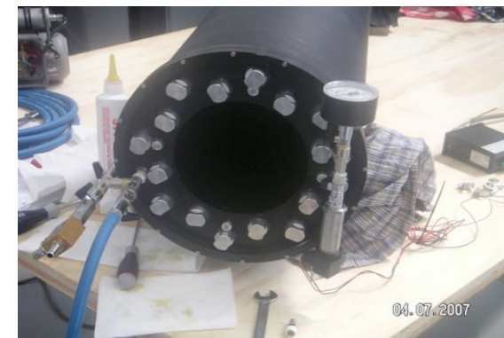
Gas pressure test
