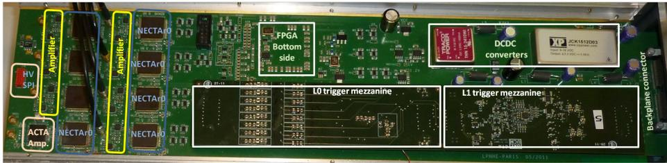
Figure 8: Global architecture of the front-end board illustrated on the FEB of the NECTAr prototype. The output of the PMTs is on the left hand side. The signal is amplified. 8 NECTAr0 chips are implemented on the FEB. The signal on 7 of these channels are equipped with commercial amplifiers. The remaining channel is equipped with an ACTA amplifier. On trigger, the data are sent to the FPGA, then to the DAQ through the backplane (on the right).
