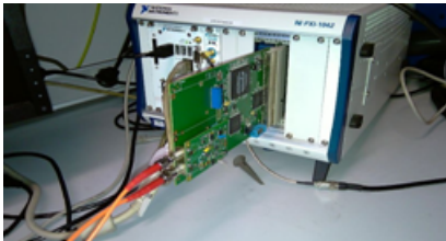
PXI crate with a MUTIN card on an extender board
