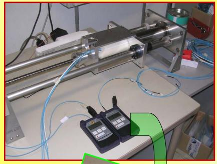
Currently the driving mechanism is under test (dry) in order to obtain a smooth operation and avoid risk of unexpected locks during wet and pressure tests.
