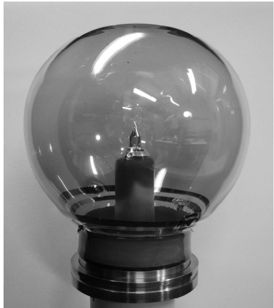
Fig. 1. Photo of the X-HPD with conical LYSO crystal anode.
