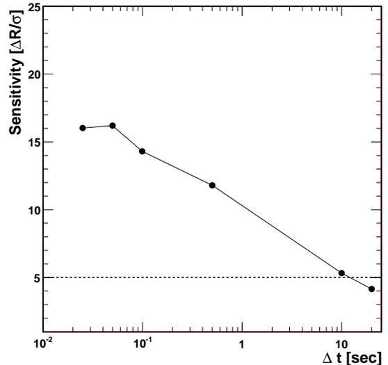
Fig. 2. Sensitivity to a supernova neutrino burst signal for different time intervals for the KM3NeT reference detector. A supernova SN1987A-type burst is assumed at a distance  $d=10$  kpc.
