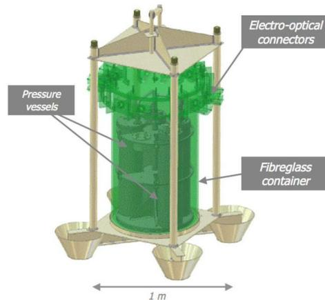
Figure 7. Junction box as used in the NEMO project.
