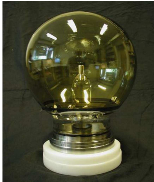
Figure 4. 8'' prototype of a spherical X-HPD tube. The development of tubes with diameters up to 15'' is planned.
