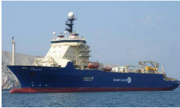
Fig. 17: A Modern DP2 Cable ship
