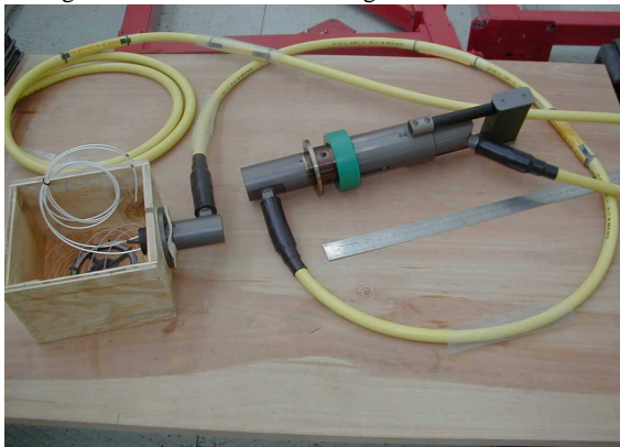
Fig. 3. A Jumper and with mated interlink cable
