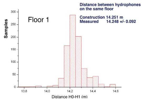
Fig. 5. Accuracy of the acoustic positioning system
