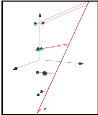
Fig. 7. Reconstruction of a downgoing atmospheric muon track.
