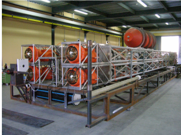
Figure 3. The NEMO prototype tower fully assembled before its deployment.
