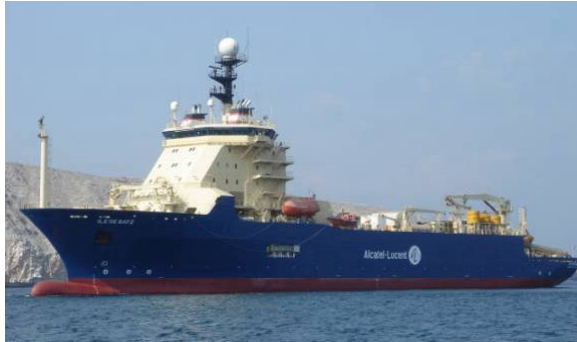
Figure 17: Modern DP2 Cable ship
