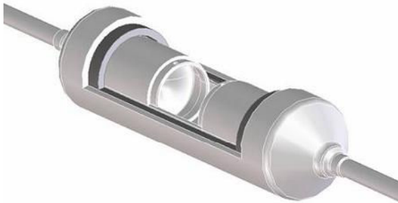
Figure 18: Deep sea cable jointing box
