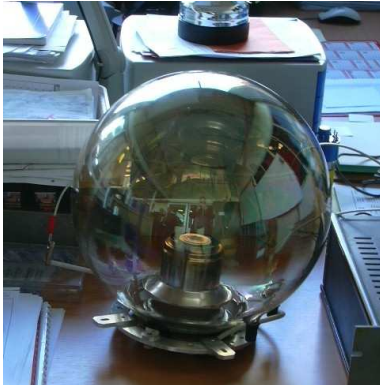
Fig. 1. The Philips XP2600 X-HPD, constructed at the Philips Brive la Gaillard site: now Photonis S.A.S
