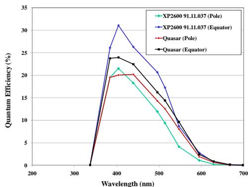
Fig. 3. Effective Q.E. gain by "double cathode" effect; polar and equatorial illumination of Quasar and XP2600 X-HPDs
