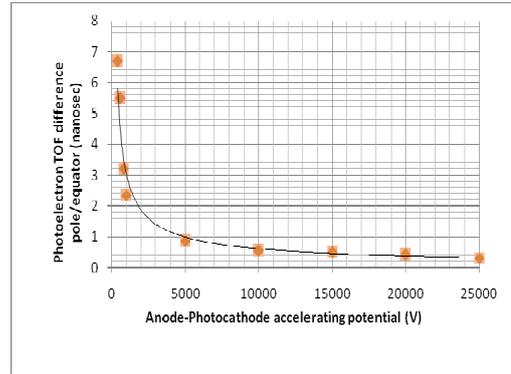
Fig. 8. Transit time difference (ns) for photoelectrons emitted at polar angles of  $0^\circ$  and  $40^\circ$ , using Simion8.
