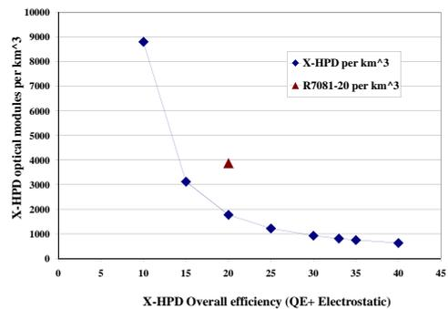
Fig. 5. N° of OMs per  $\text{km}^3$ , comparing the Hamamatsu 10" R7081-20 PM of ANTARES with same diameter X-HPDs of  $3\pi$  solid angle coverage and overall efficiency up to 40%.
