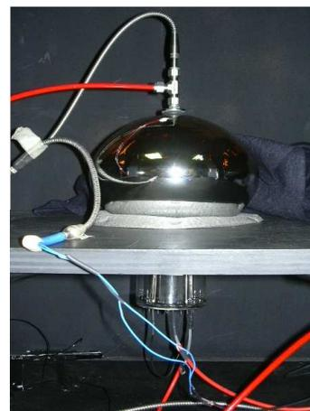
Fig. 6. X-HPD envelope demonstrator: all-glass construction with internally-processed bialkali photocathode.
