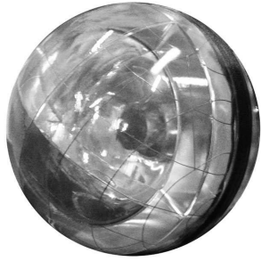
Fig. 5. The complete Directional Optical Module ready to be tested. The mu-metal cage and the mirror system are visible.
