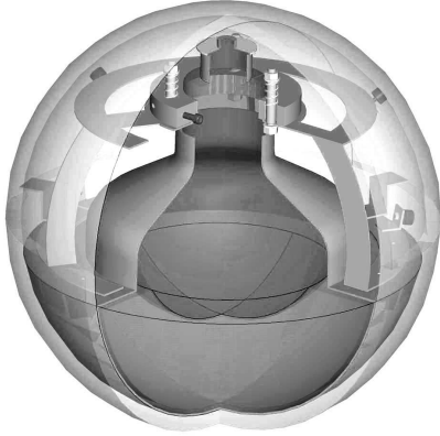
Fig. 1. A section of a directional OM: if compared to a traditional one, the thick light guide with mirrors is the main difference.
