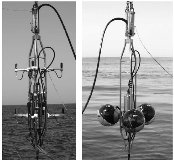
Fig. 3. Storey 3 of the IL07 (left) and Storey 21 of L12 (right) during their deployment.
