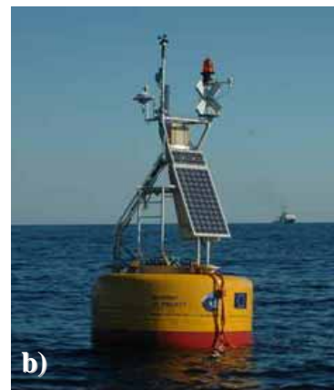
Fig. 2. Images of: a) GEOSTAR seafloor observatory (bottom) and MODUS (top); b) relay surface buoy for the communications
