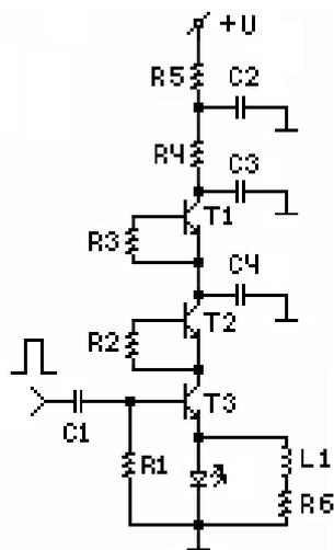
Fig.6. Scheme of a powerful nanosecond light source based on a single high power blue LED – LXHL-NB98.
