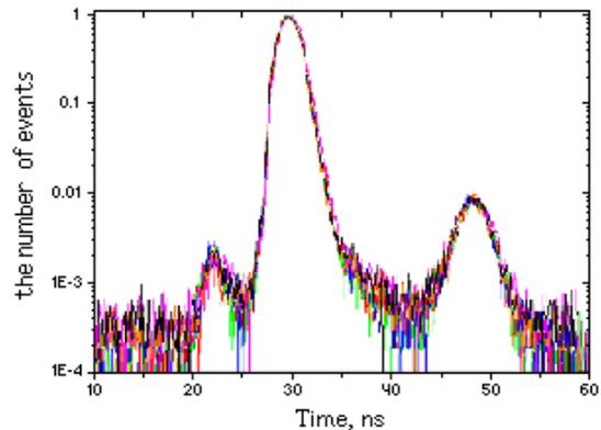
Fig.4. Light emission kinetics of the LED matrix (the black curve) and individual LEDs of the matrix (the colored curves). The “one driver – a matrix of LEDs” approach.
