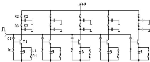
Fig.1. Scheme of a powerful nanosecond light source based on the matrix of LED drivers. The “one LED – one driver” approach.
