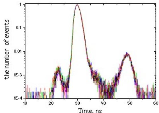
Fig.2. Light emission kinetics of the LED matrix (the black curve) and individual LEDs of the matrix (the colored curves). The “one LED – one driver” approach.
