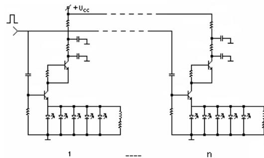
Fig.5. Cluster of  $n$  matrixes of LEDs.
