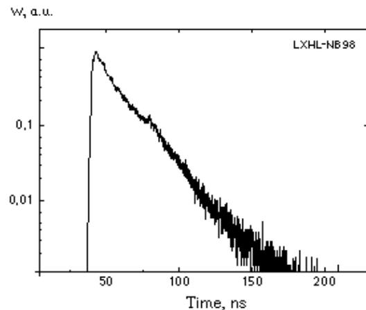
Fig.7. Typical light pulse shape of a single high power blue LED (LXHL-NB98 from LUMILED).
