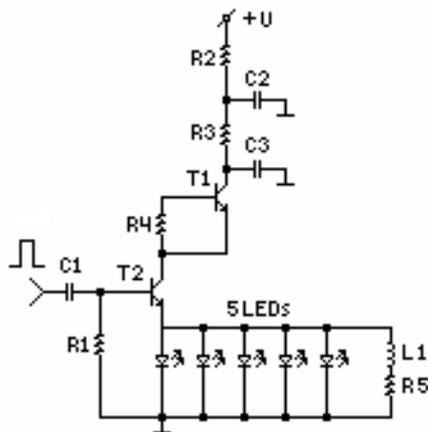
Fig.3. Scheme of a powerful nanosecond light source based on the matrix of LED. The “one driver – a matrix of LEDs” approach.
