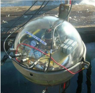
Fig. 9. An OM with phototube XP1807 after final mounting
