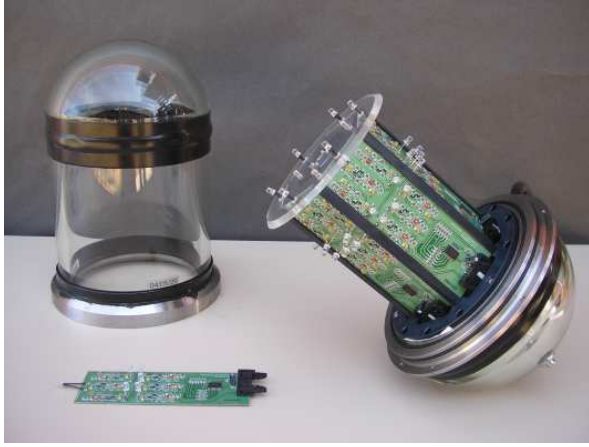
Fig. 2. View of the LED Optical Beacon used in ANTARES. The picture shows the hexagonal frame with the 36 LEDs, and the glass container devised to protect the device under-sea.
