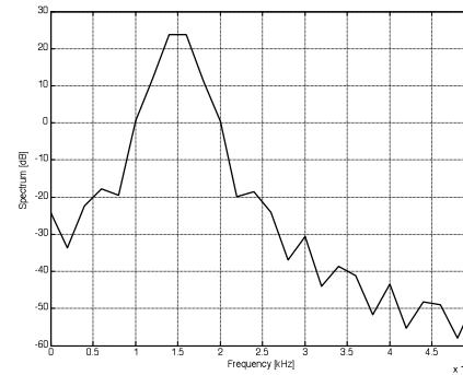
Transmitted burst and waveform spectrum (logarithmic scale, arbitrary reference)
