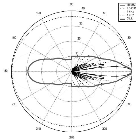
Composite beampattern of a click, created by applying its estimated power spectral density to a 0.8 m circular transducer that creates forward beams only from 5kHz upwards, and bidirectional beams downwards. The resulting click DI is 21.3 dB
