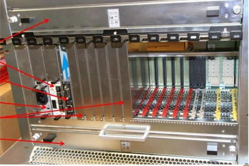
12 Payload AMC-RTMs **Dual Star Redundant** Front View
