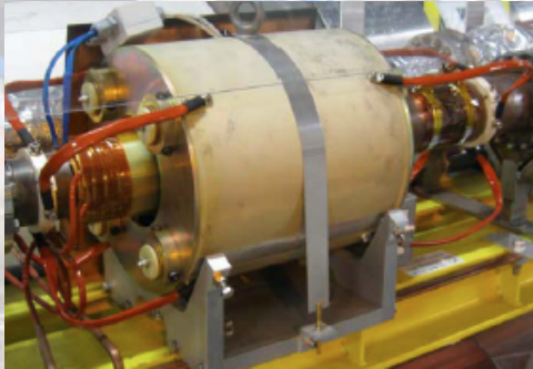
Direct-Current Current Transformer (DCCT) (measure the total current)
