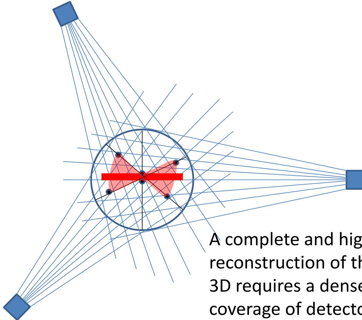
A complete and high resolution reconstruction of the image in 3D requires a dense azimuthal coverage of detectors
