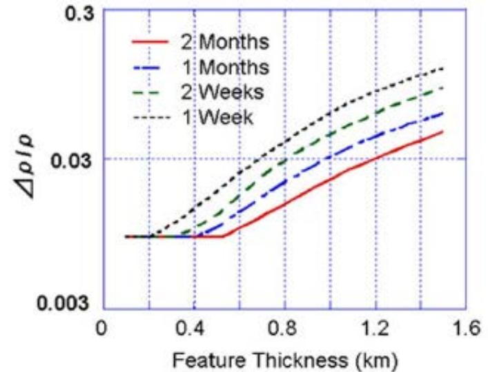
The figure summarizes the tradeoff between observation time and density contrast for features to be resolved to within one standard deviation with a detector with area of 4000 cm<sup>2</sup> located about 1 km from the target (Tanaka et al 2007).
