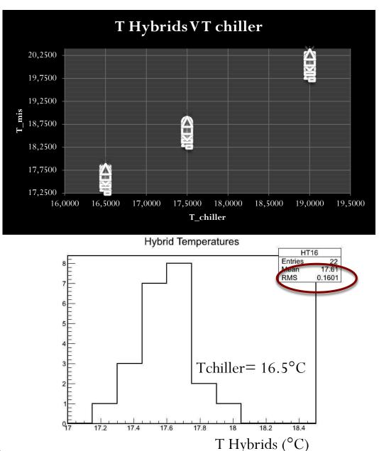
..and excellent uniformity of all hybrids' temperatures for a given value of T (RMS = 0.16 °C)
