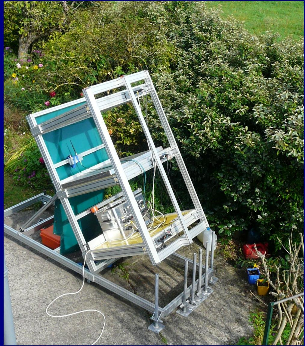
One of the 4 telescopes in a 3-matrices + shielding configuration during acceptance calibration experiment
