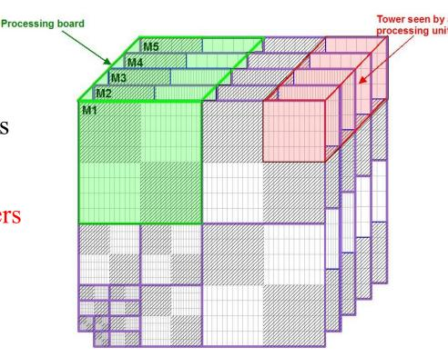
All towers contain the same quantities of data to analyse but cover a smaller area near the beam axis because the higher density of pads.
