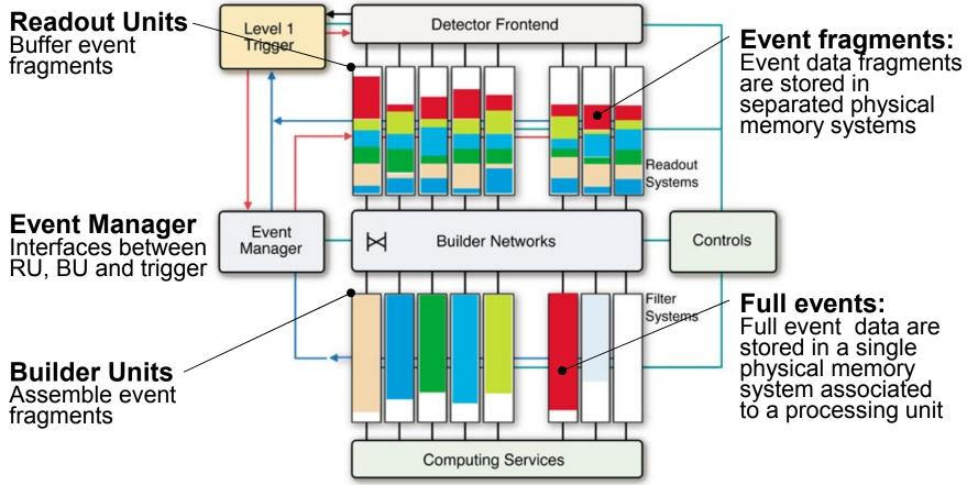
Requirements: L1 trigger: 100 kHz (@2KB), ev-size 1MB, 200 MB/s in AND out per RU, 200 MB/s in AND 66 MB/s out per BU
