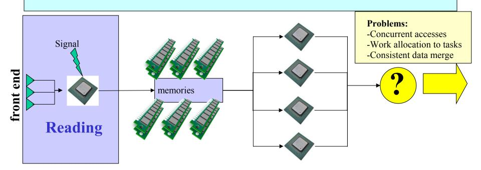
If stable input flow And limited by processing time Then add more processing units to work in parallel (example read DMA engine, use multiprocessor or multicore for analysing tasks)
