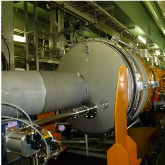
Capture Cryomodule (two 9-cell cavities) 2012', Feb. Cool-down
