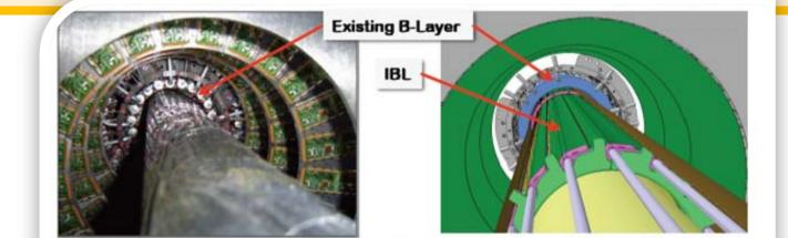
Mission impossible... fit an additional layer in between Pixel and beam-pipe: · Reduce beam-pipe by 4 mm in radius... and make it possible! <r>=33 mm vs present <r<sub>min</sub>> = 50.5 mm
