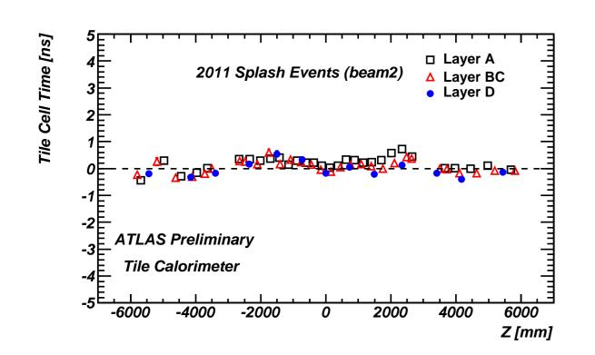
During special single-beam runs, the beam reaches a closed collimator near the ATLAS detector; the resulting event is called a *splash event*; splash events are used to evaluate the TileCal timing, after corrections have been applied for particle time-of-flight and fiber length. The TileCal cell synchronization is over the whole calorimeter within 1 ns.
