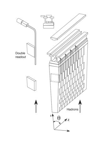
TileCal is made of steel and scintillating tiles coupled to optical fibers and read out by photomultipliers. The WLS fibers are coupled to form cells of about  $0.1 \times 0.1$  in  $\Delta \eta \times \Delta \phi$ .
