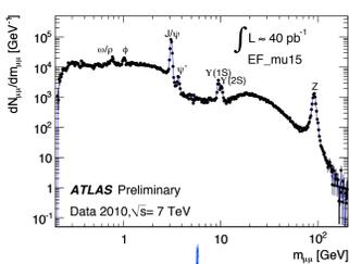
The  $J/\psi \rightarrow \mu^+\mu^-$  decay is used to obtain a sample of low- $p_T$  probes, while the  $Z \rightarrow \mu^+\mu^-$  decay provides high  $p_T$  probes
