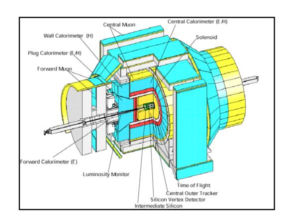
• Time-of-flight detectors provides particle ID
