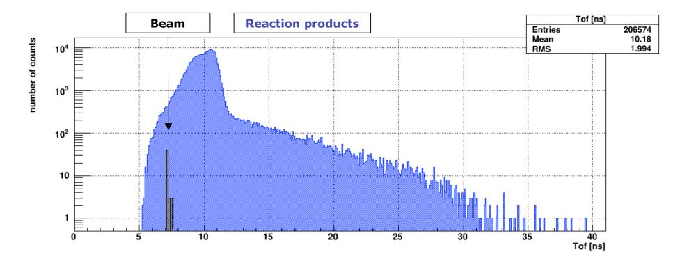
Time-of-flight spectra of beam and reaction products at the distance of 20 cm from target
