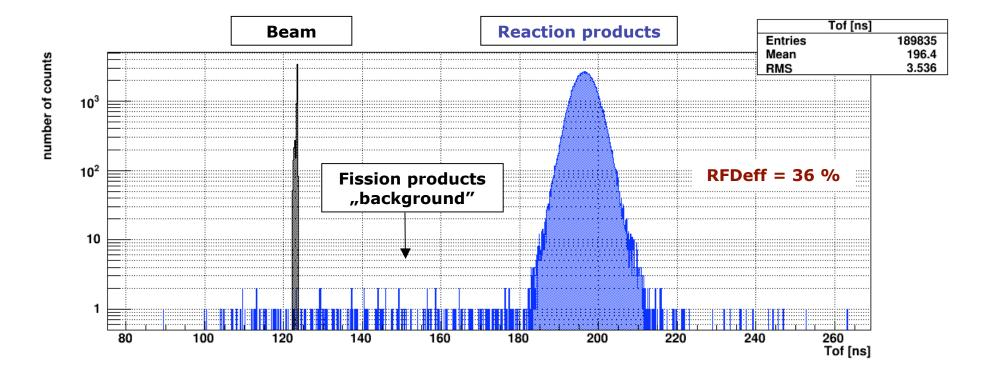
Time-of-flight spectra of beam and reaction products at the distance of 3.5 m from target
