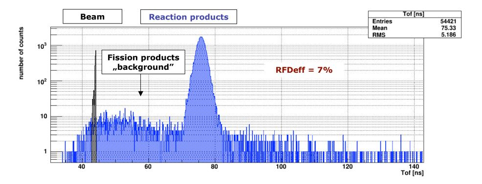
Time-of-flight spectra of beam and reaction products at the original distance of 1.25 m from target
