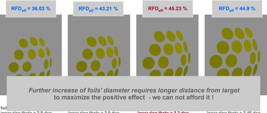
inner ring theta = 2.9 deg middle ring theta = 5.1 deg outer ring theta = 5.69 deg distance from target = 3.5 m inner ring theta = 2.9 deg middle ring theta = 5.1 deg outer ring theta = 5.9 deg distance from target = 3.5 m inner ring theta = 3.2 deg middle ring theta = 5.65 deg outer ring theta = 6.55 deg distance from target = 3.5 m inner ring theta = 3.45 deg middle ring theta = 6.0 deg outer ring theta = 7.0 deg distance from target = 3.5 m
