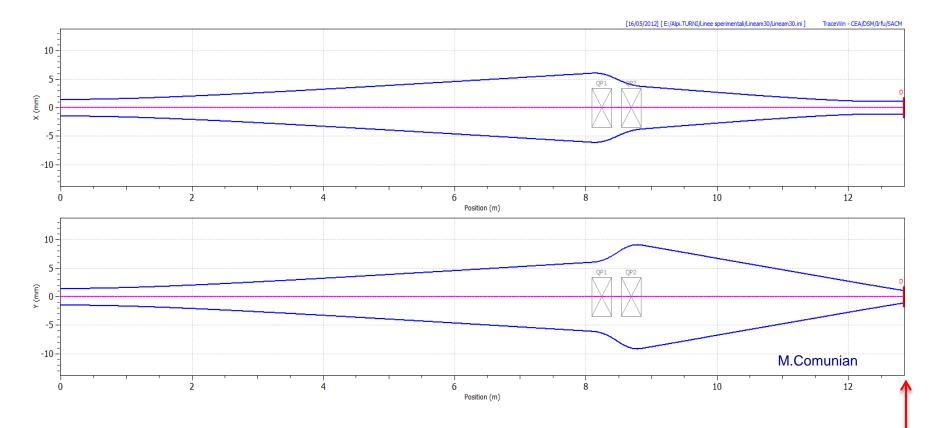
Ion optics calculations performed by the accelerator division at LNL beam envelope in X (top) and Y (bottom) directions
