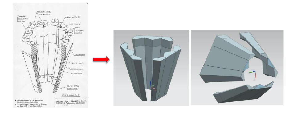
□ a proposal for the construction of the triple cluster AC shield out of the individual crystals of the original EB cluster shield
