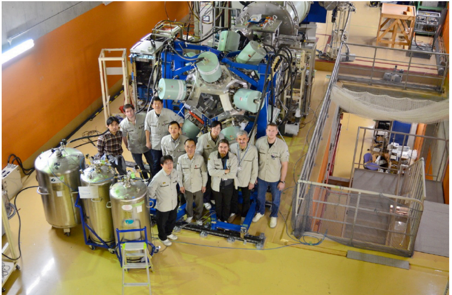
EURICA installed at focal plane of Big RIPS separator.
