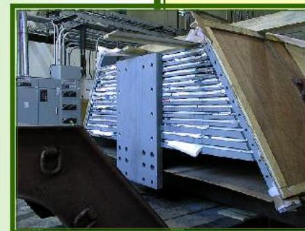
Barrel RPCs Loaded Into Flux Return
