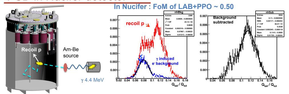
→ configuration of the Nucifer vessel preserves an e-p separation at quasi same level than in small test cell.
